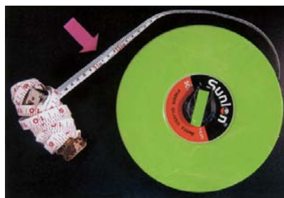
量度短樁用的「神仙尺」 Rigged measuring tape used for measuring shortened piles
